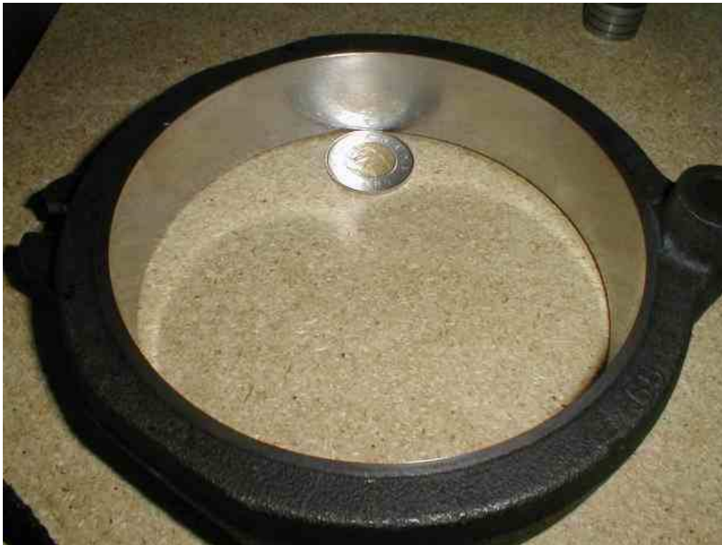
Can ring machined and sanded
