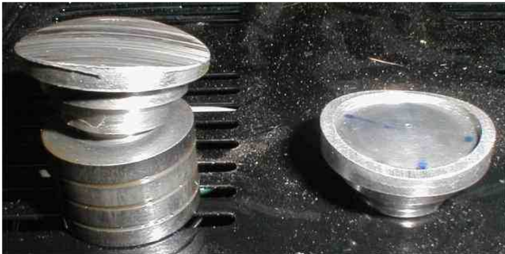
Worn and new (used) slippers
