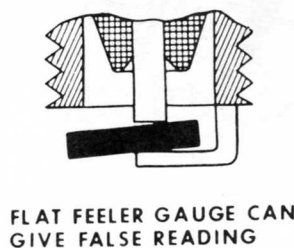
FIGURE 42. SPARK PLUG GAP
