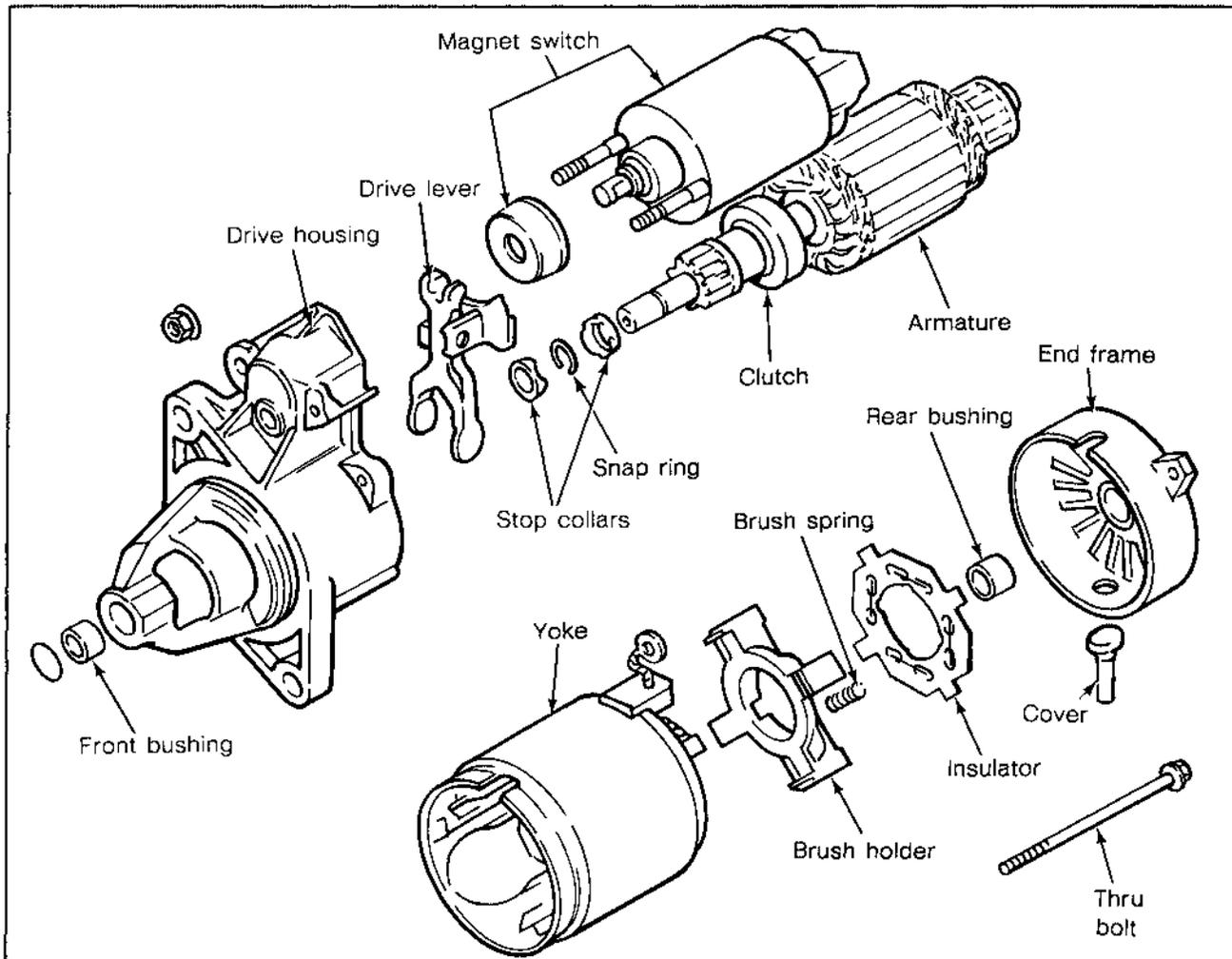
Figure 8-21. Exploded View of Nippendenso Solenoid Shift Starter.
