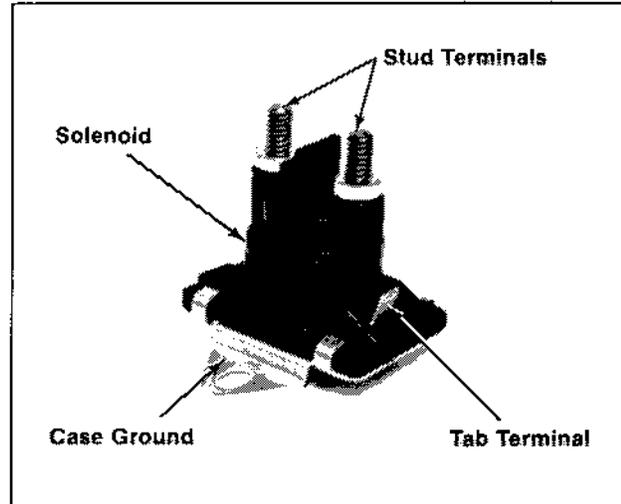
Figure 8-16. Starter Solenoid.
