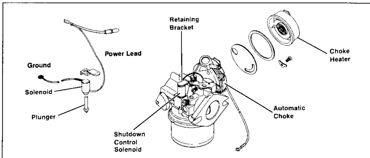
**Figure 6A-23. Engine Shutdown Control and Automatic Choke.**
