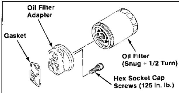
Figure 7-6. Installation Torques--
