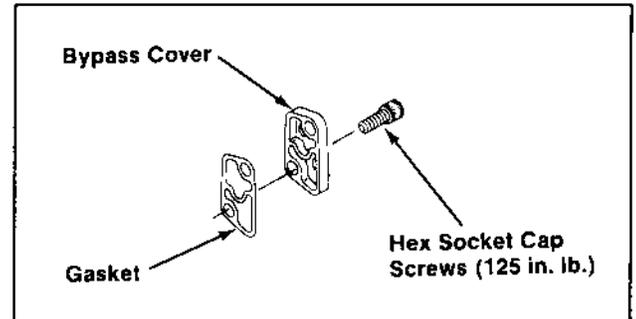
Figure 7-7. Installation Torque--Filter Bypass Cover
