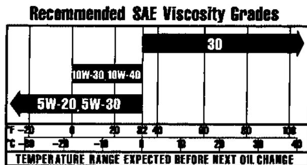
Straight 30-weight oil is preferred. SAE 10W-30 and 10W-40 are not recommended above 32°F (0°C). Using these oils substantially increases oil consumption and combustion chamber deposits.
