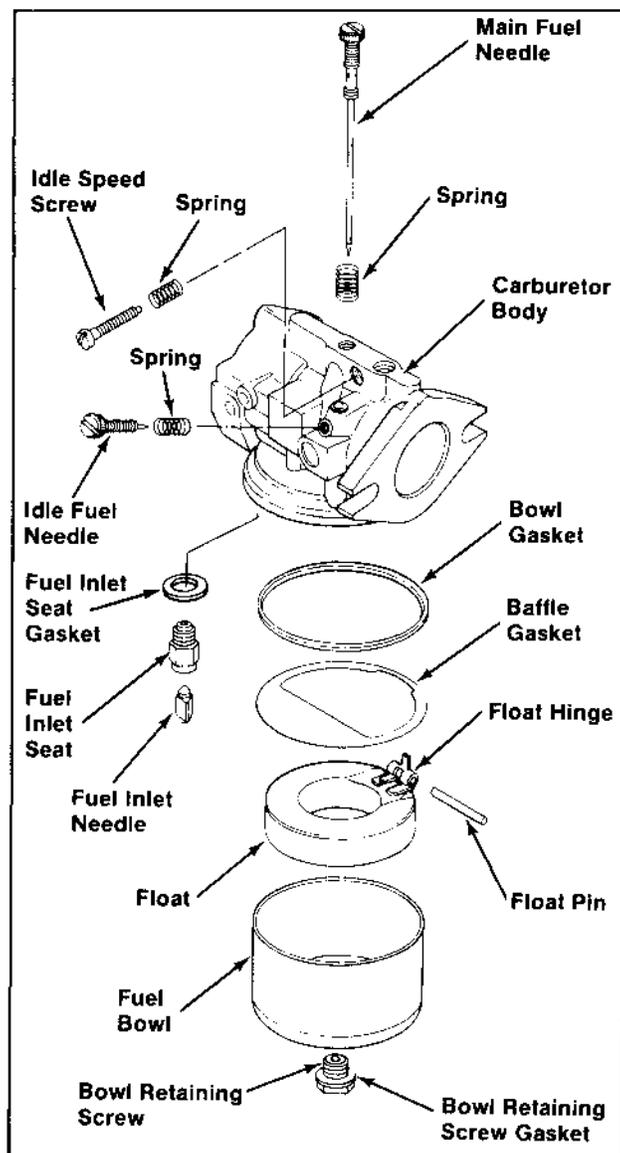
Figure 6A-7. Kohler-Built Adjustable Jet Carburetor – Exploded View.
