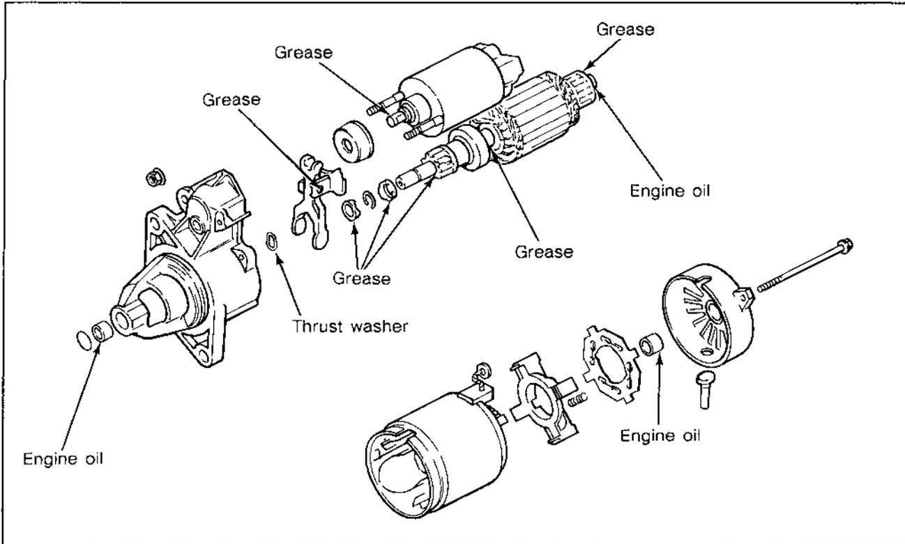
Figure 8-34. Lubrication Points.
