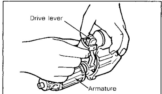
Figure 8-23. Removing the Armature and Drive Lever.
