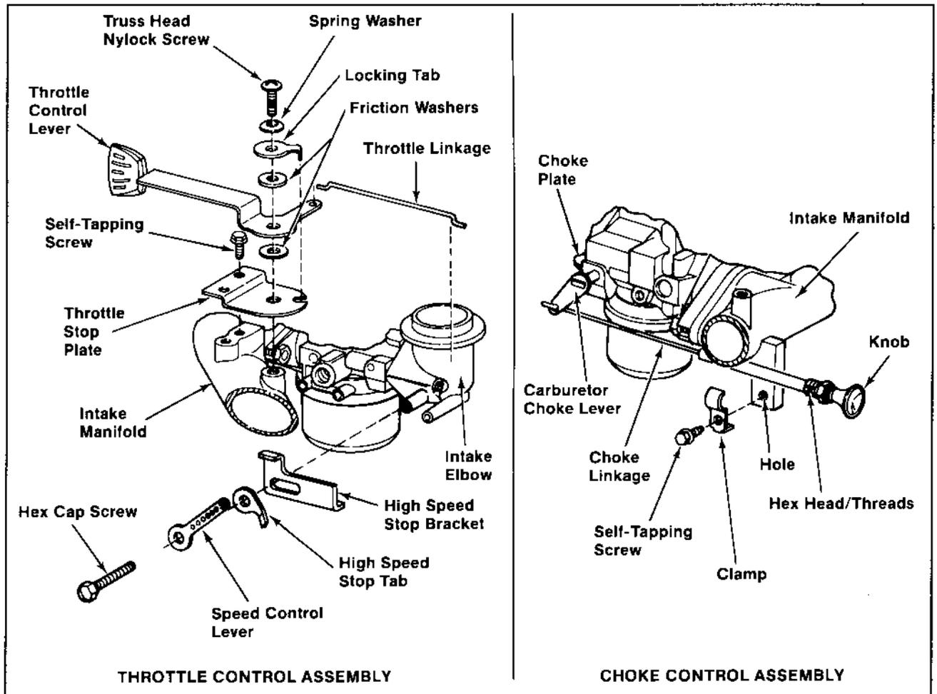
Figure 6A-21. Engine Mounted Throttle and Choke Controls.
