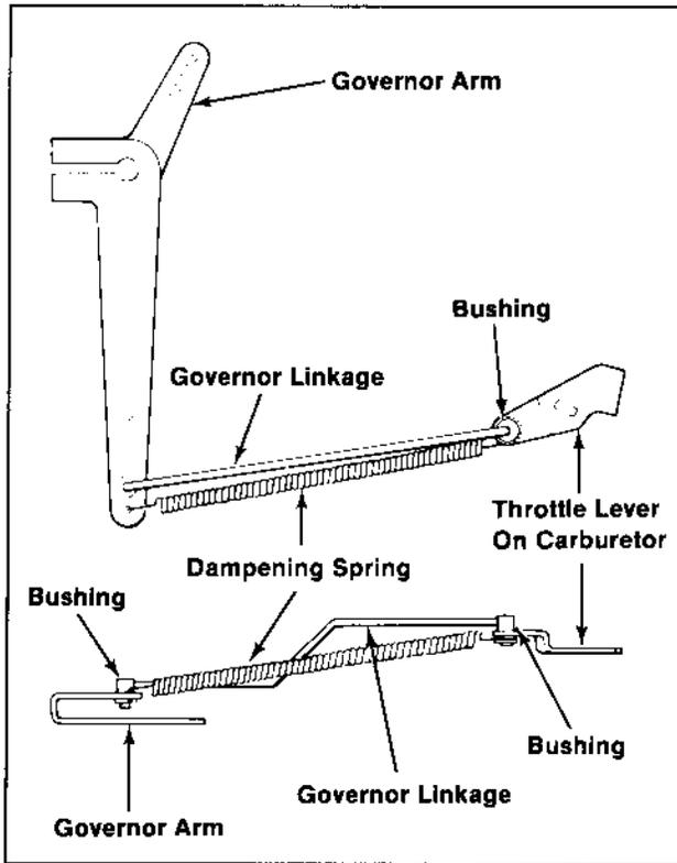
Figure 6B-16. Installing Dampening Spring --
