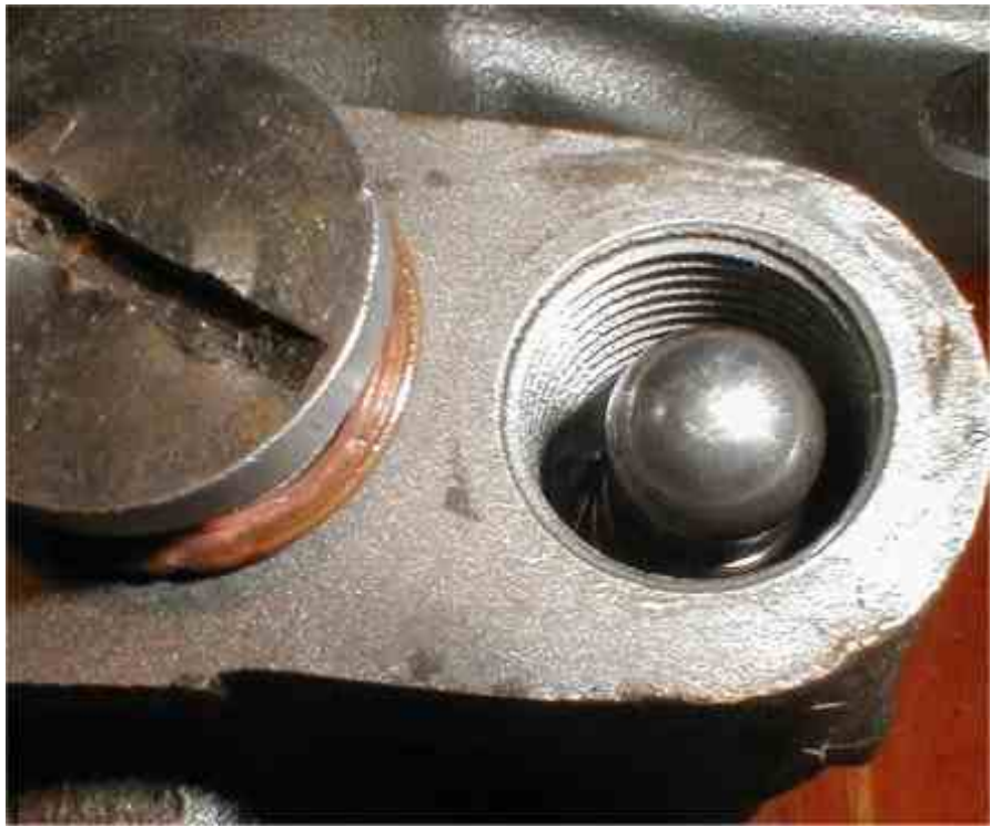
Check ball & spring for the P-N-D oil bypass
