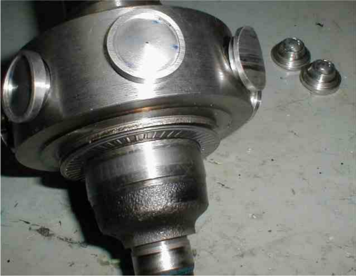
Radial pump with new (used) and worn slippers
