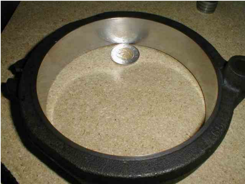
Can ring machined and sanded
