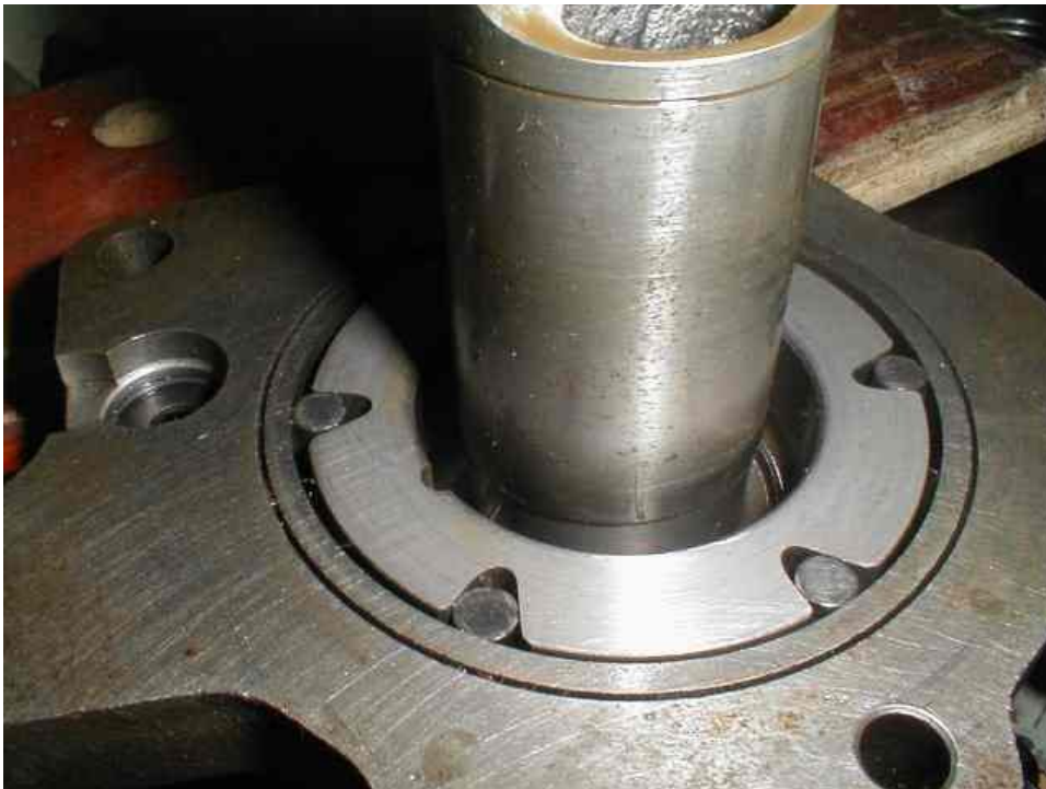
Six rollers pins 1/4 X 9/16
