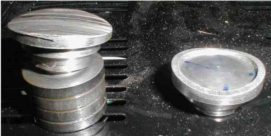
Worn and new (used) slippers
