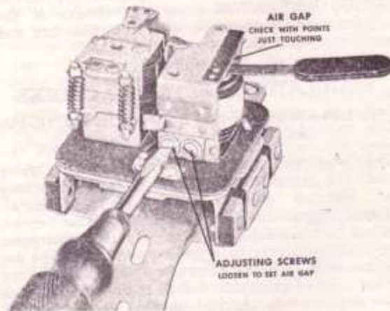
Figure 7—Cutout relay air gap check and adjustment (1118200 series). Battery must be disconnected when this check is made.
