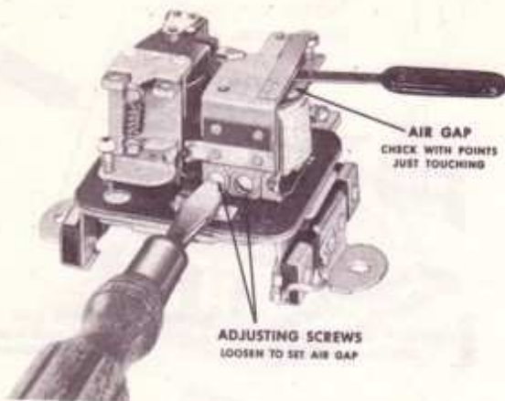
Figure 8—Cutout relay air gap check and adjustment (1118300 and 1118700 series). Battery must be disconnected when this check is made.
