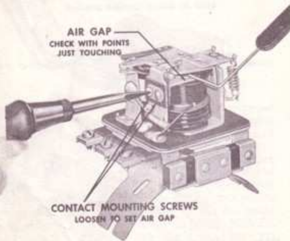
Figure 13—Current-voltage unit air gap check and adjustment (1118200 series).
