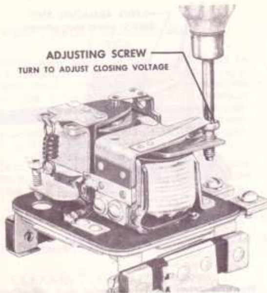
Figure 12—Adjustment of cutout relay closing voltage (1118300 and 1118700 series).
