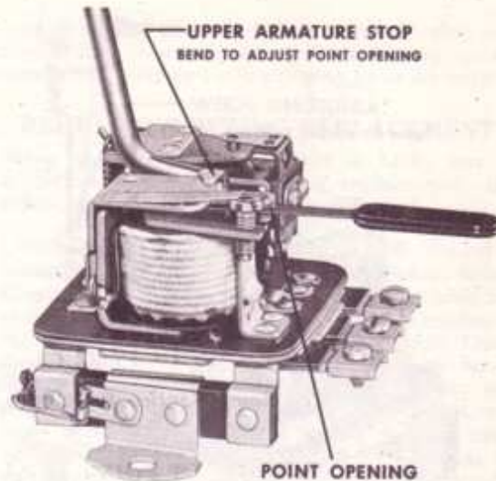
Figure 10—Cutout relay point opening check and adjustment (1118300 and 1118700 series). Battery must be disconnected when this check is made.
