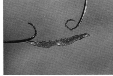
Pinching of the O-ring seal will occur if it's not properly placed in its groove.
