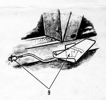
9. Remove foot rest and disconnect brake linkage at rear by removing cotter pin. Install foot rest braces using existing bolts (on right hand side foot rest brace to slide over brake linkage). Reinstall foot rest and reconnect brake linkage.
