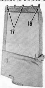
16. Insert bent strap into front hem of door. Attach clip using 3/16 x 1/2 slotted screw and nut. (Bulge in clip and head of screw toward outside of door.)
