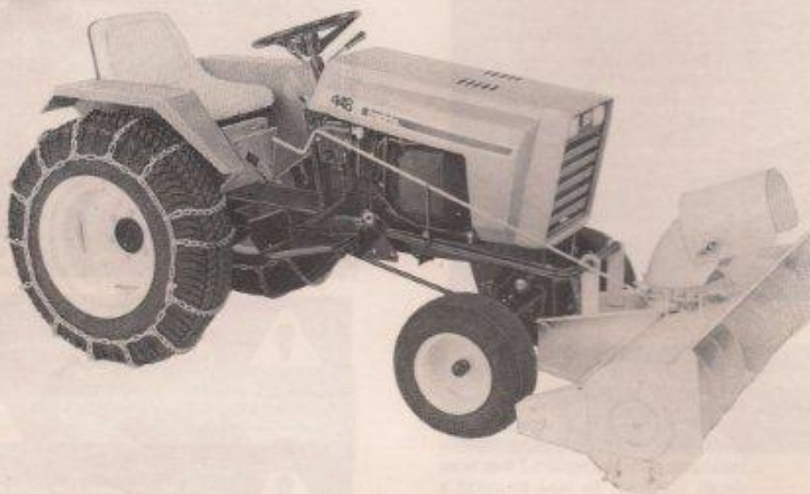
FIGURE 1 Tractor with Snow Caster, Rear Weight Kit, Tire Chains and Flow Control Valve
