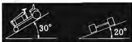
The diagram depicts the maximum angles that the stationary tractor, less mounted equipment, was subjected to without tipping, measured on a perfectly flat, smooth, and hard surface. This illustration does not recommend safe operating limits as the slope, type of terrain and all applicable factors as discussed in this manual must be taken into consideration by any person whenever operating the tractor.
