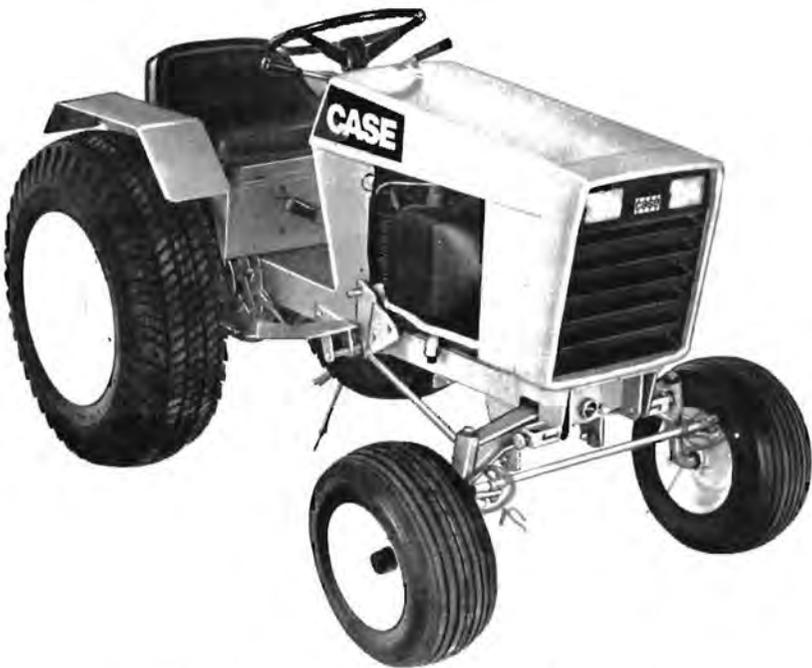
**FIGURE 2. Right Hand View of Case 446 Compact Tractor**
