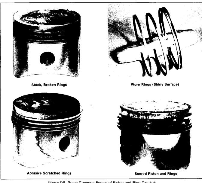
Figure 7-8. Some Common Forces of Piston and Ring Damage
