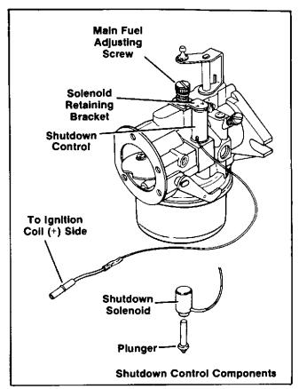
Figure 4-4. Engine Shutdown Control
