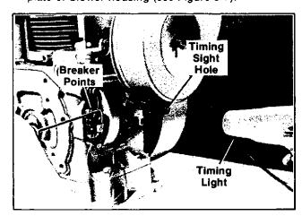
Figure 5-7. Timing Light Method
