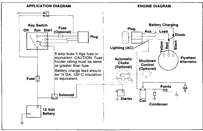
Figure 5-9. 3/6 Amp System Wiring Diagram
