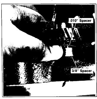
Figure 8-1. Installing Balance Gears
