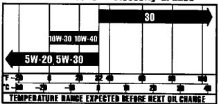
Use straight weight oils as specified. Do not use multi-viscosity oils above 32°F as considerable increases in oil consumption and combustion deposits will result.
