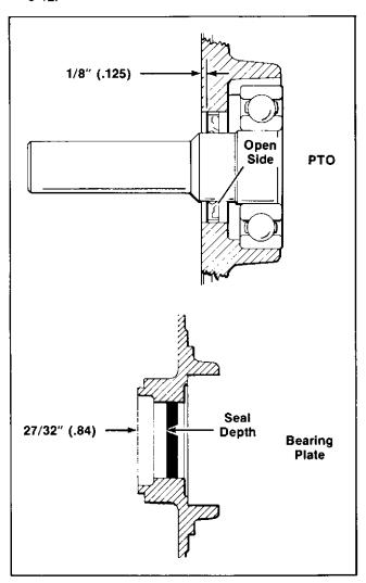
Figure 8-12. Drive Oil Seal to Specified Depths
