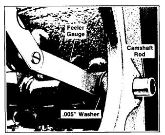
Figure 8-3. Checking Camshaft End Play
