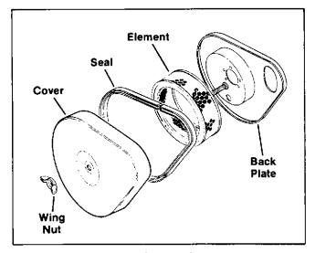
Figure 3-1. Air Cleaner Components
