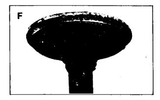
Coking: Coking, as shown in View F, is normal on intake valves and is not harmful. If the seat is good, this valve could be reused after cleaning.
