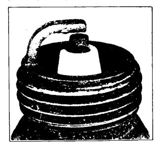
Overheated: Overheating will be indicated by chalk white colored deposits, not burned black as might be expected. This condition is also usually accompanied by excessive gap erosion. Overadvanced timing, lean carburetion, clogged air intake and blocked cooling fins are some of the causes of overheating.
