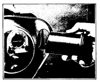
Figure 8-26. Installing Air Cleaner Back Plate and Tube
