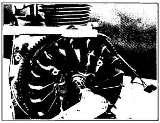
Figure 8-18. Torquing Flywheel
