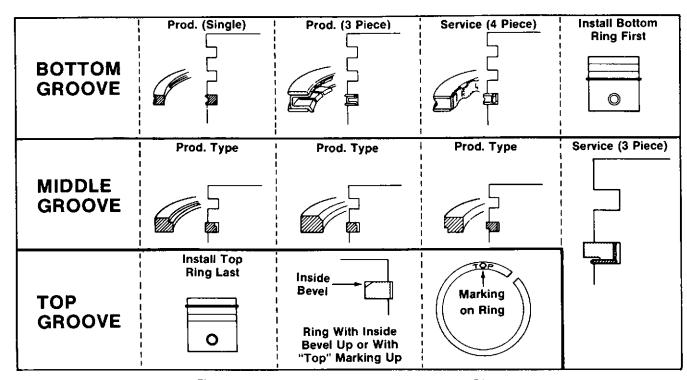
Figure 7-10. Production Type and Service Type Rings
