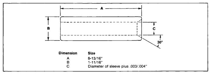
Figure 9-3. Dimensional Diagram - Seal Driver
