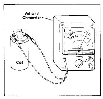
Figure 5-3. Continuity Check in Primary of Coil
