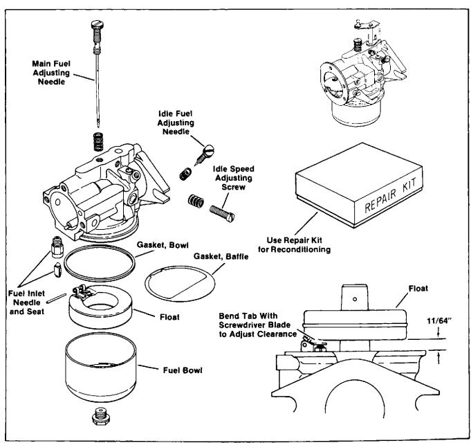
Figure 4-2. Side Draft Carburetor
