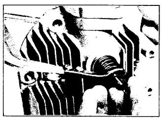
Figure 8-13. Installing Valve Springs
