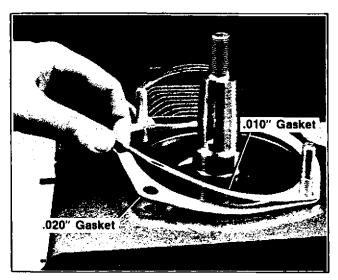
Figure 8-7. Installing Gaskets for Crankshaft End Play
