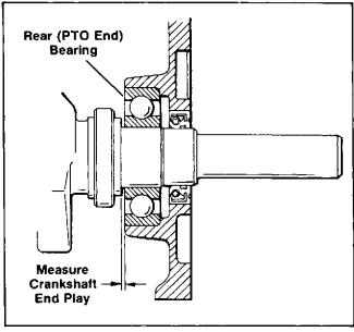
Figure 8-8. Measuring Crankshaft End Play
