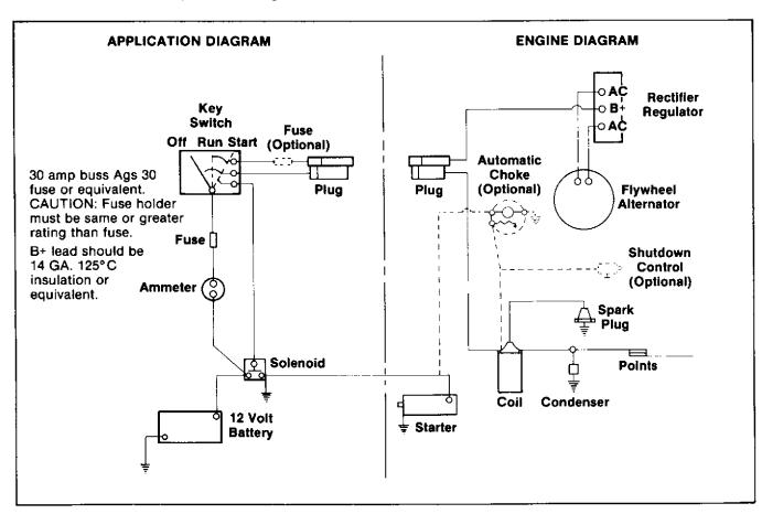
Figure 5-10. 15 Amp System Wiring Diagram
