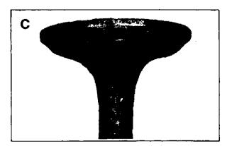
Stem Corrosion: Moisture in fuel or from condensation are the most common causes of valve stem corrosion as shown in View C. Condensation occurs from improper preservation during storage and when the engine is repeatedly stopped before it has a chance to reach normal operating temperatures. Replace corroded valves.
