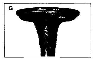
**Gum:** Gum deposits usually result from using stale gasoline. This condition is often noted in applications where fuel is not drained out of tank during the off season. Also check carburetor if gummy substance is found on the valve stem. Gum is a prevalent cause of valve sticking. The cure is to ream the valve guides and clean or replace the valves, depending on their condition.
