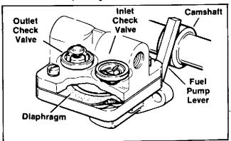
Figure 4-5. Fuel Pump Function
