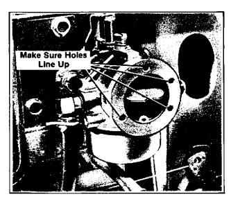
Figure 8-25. Carburetor Air Horn Gasket Installed
