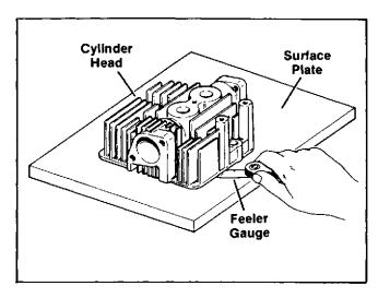
Figure 7-4. Checking Cylinder Head Flatness
