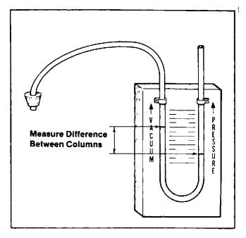
Figure 2-1. "U" Tube Water Manometer
