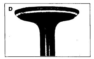
Overheating: An exhaust valve subject to overheating will have dark discoloration in area above valve guide. Worn guides and faulty valve springs may cause this condition. Also check for clogged air intake, blocked fins, and lean fuel mixture when this valve condition is noted.
