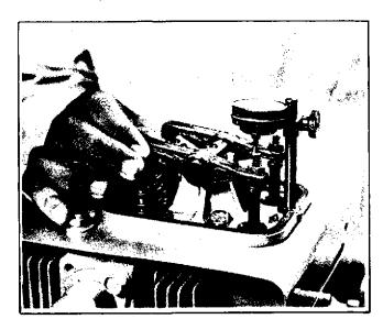
Figure 6-2. Checking ACR Function
