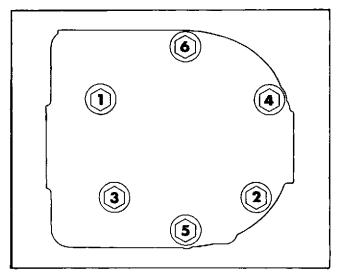
Figure 9-1. Headbolt Torque Sequence
