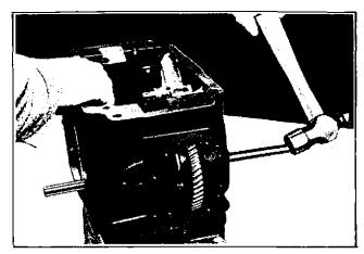
Figure 7-12. Camshaft Removal
