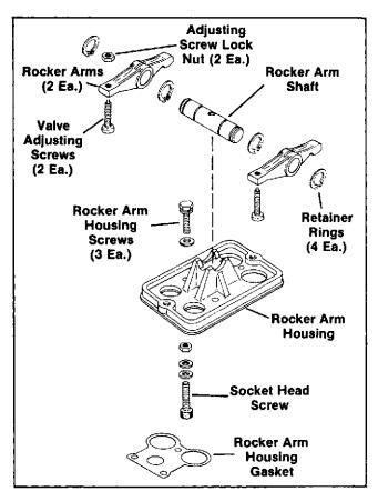
Figure 8-15. Rocker Arm Assembly
