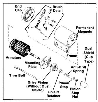
Figure 5-11. Exploded View of Typical PM Starter
