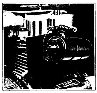
Figure 8-22. Securing Coil and Condenser to Side Baffle
