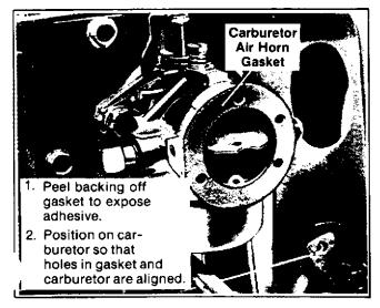
Figure 3-2. Air Horn Gasket Installation
