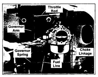
Figure 8-23. Connections to Carburetor (Throttle, Fuel and Governor)
