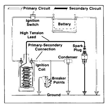
Figure 5-1. Schematic of a Typical Battery Ignition System
