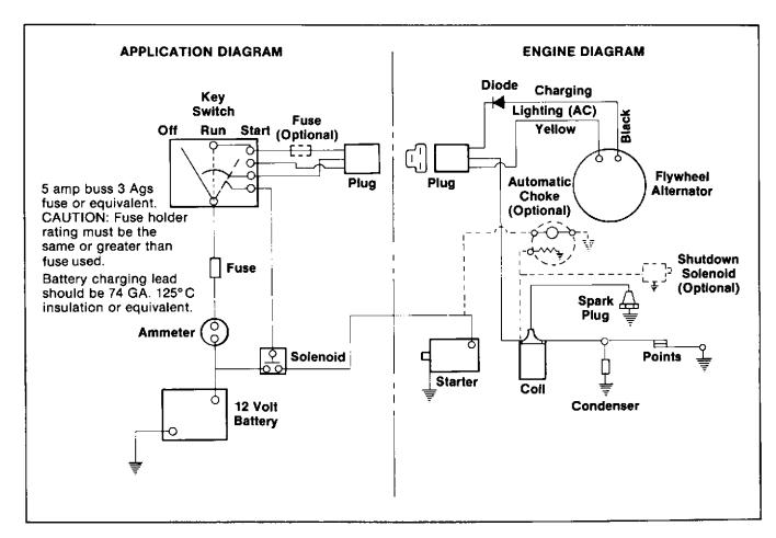
Figure 5-8. 3 Amp System Wiring Diagram
