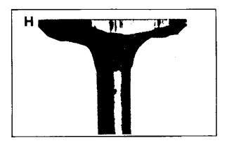
Carbon Cut: Excessive build-up of carbon in the combustion chamber may result in valve damage as shown in View H. Carbon can become hard enough to cut the valve. Cleaning of the cylinder head at proper intervals could prevent such damage.
