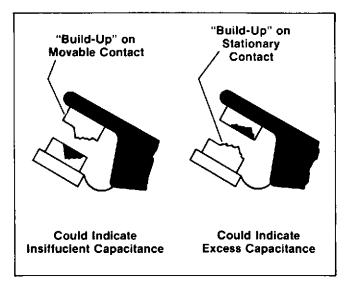
Figure 5-2. Metal Transfer on Points
