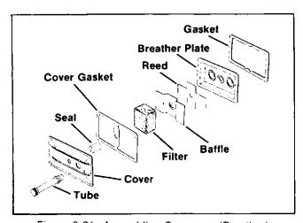
Figure 8-21. Assembling Sequence (Breather)
