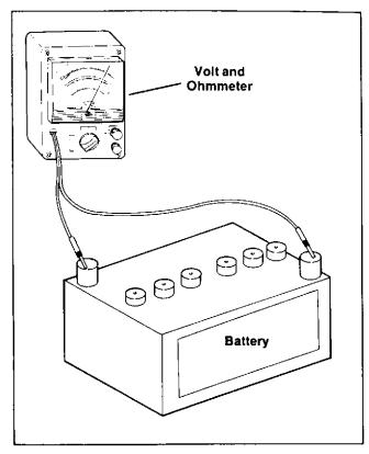
Figure 5-5. Checking Battery Charge
