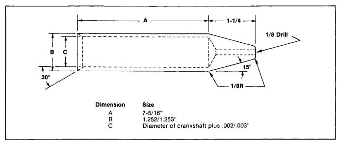
Figure 9-2. Dimensional Diagram - Seal Sleeve
