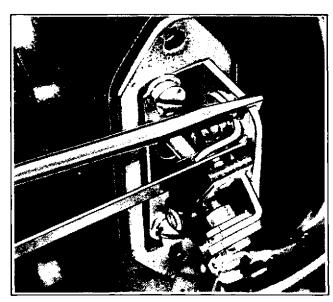
Figure 5-6. Point Gap Adjustment
