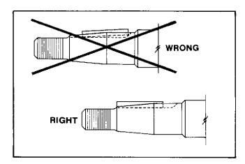
Figure 8-17. Right and Wrong Way to Install Flywheel Key
