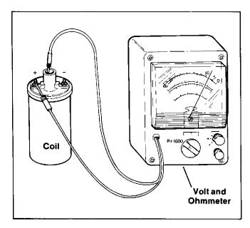
Figure 5-4. Resistance Check in Secondary of Coil
