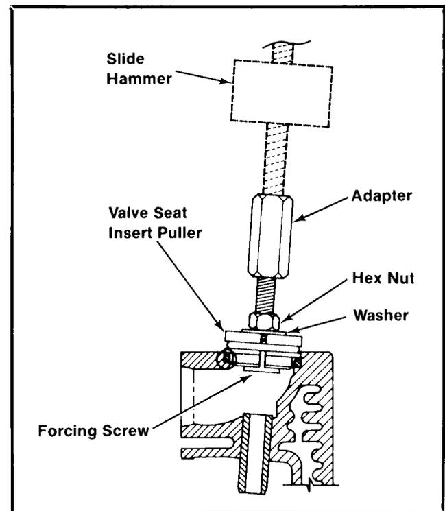
**Pulling Valve Seat Insert (Typical)**
