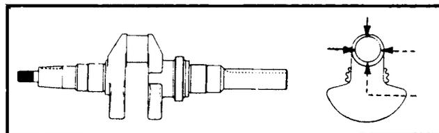
NOTE: If the crankpin is reground, visually check to insure that the fillet blends smoothly with the crankpin surface.
