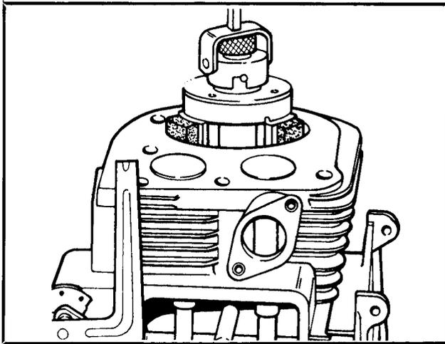
1. Lower hone into bore and after centering, adjust so that stones are in contact with walls. Use of a commercial cutting/cooling agent is recommended.
