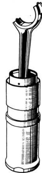
FIGURE 29. INSTALLING PISTON ASSEMBLY IN SLEEVE
