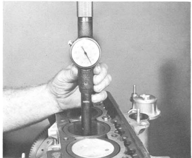
FIGURE 17. CHECKING I. D. OF SLEEVE BORE
