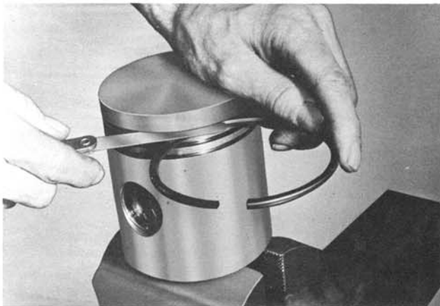
FIGURE 25. CHECKING RING CLEARANCE IN GROOVE
